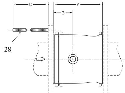
Figure 4. Required clearances for installation of design CVS V-100 Ball Valve Body
