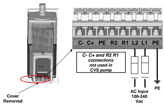
Internal Power Terminal Block Connections
