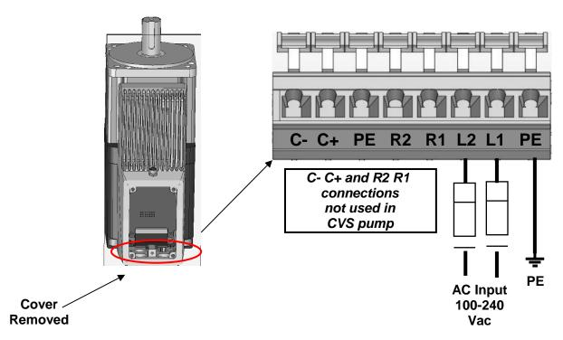
Internal Power Terminal Block Connections
