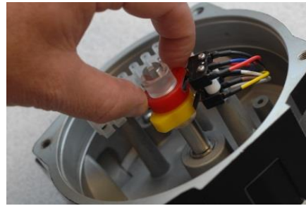
Red Cam Adjustment – Fully Closed
