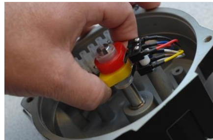
Yellow Cam Adjustment – Fully Open
