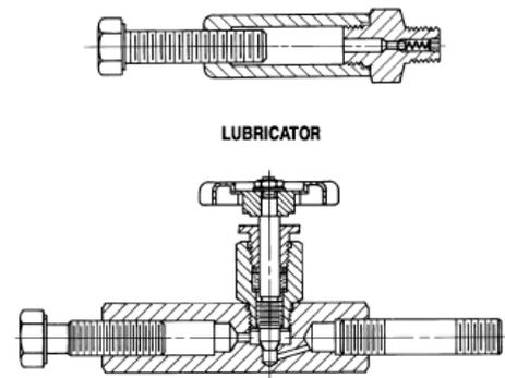
Figure 2: Optional Packing Lubricator, and Lubricator Isolating Valve
